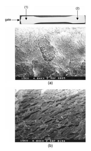
Fig. 9. Cross sectional morphologies of blends obtained at two different sampling positions 1 and 2 when blend contains PMMA as compatibilizer: (9-a): position 1, (9-b): position 2.
