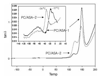
Fig. 5. Dynamic mechanical behavior (tan d) of PC/ASA-1 and PC/ASA-2 blends.
