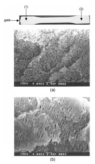
Fig. 8. Cross sectional morphologies of blends obtained at two different sampling positions 1 and 2 when blend contains TMPC-b-SAN copolymer as compatibilizer; (8-a): position 1, (8-b).
